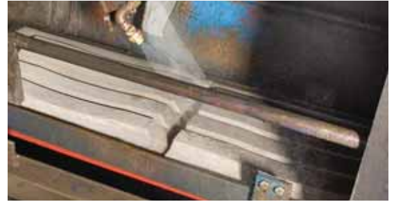
The tile mold release oil purchased is recycled from restaurant fryers. The oil is vegetable based.
