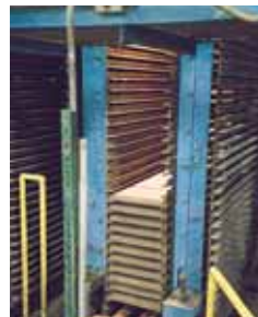
A low-NOx process is employed in our tile curing chambers.
