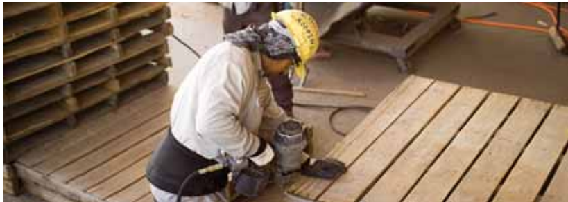
Wood tile pallets are repaired and re-used whenever possible.
